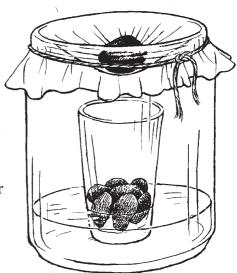
Tie a dry plastic sheet over the mouth of the larger container. A stone at the centre of the sheet should make it slope into the smaller container.
